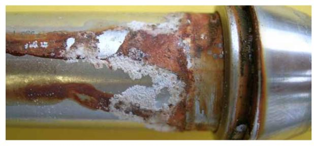
**Failure approaches** — **in just 7 days!** This image shows corrosion around a tube fitting assembly after just 175 hours exposure to salt spray (as per ASTM B117), a common problem in offshore environments. The tubing itself — also sourced from a low cost producer — is corroding just as rapidly.
